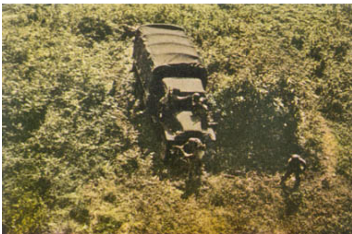
FIGURE 48. A sloped side screen hung from a tree conceals a vehicle from oblique observation. Repairs, unloading, and other activities can be carried on behind it. Camouflage nets used as drapes can often combine the principles shown in figures 47 and 48, and thus provide concealment from both ground and air observation.
